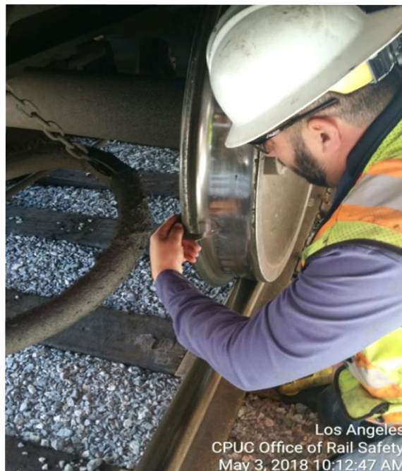
CPUC MP&E inspector measuring a wheel flange
