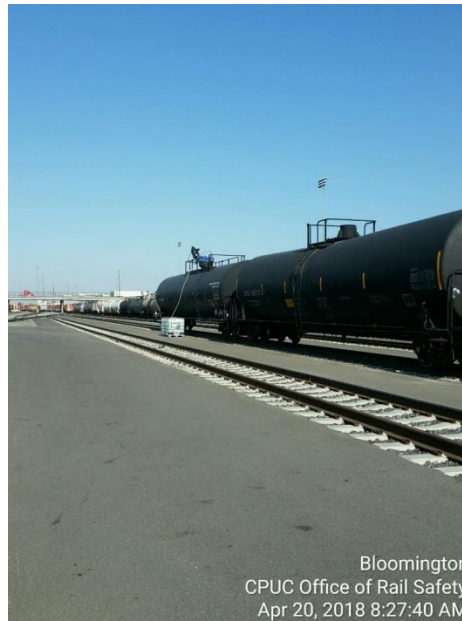
Vapor control system attached to sample line of the anhydrous ammonia car
