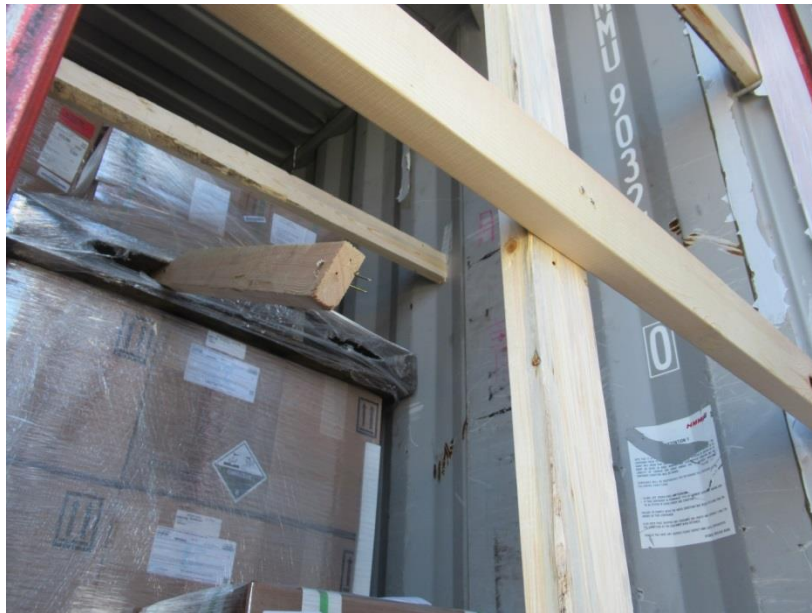
Failed blocking and bracing of hazardous materials containers
