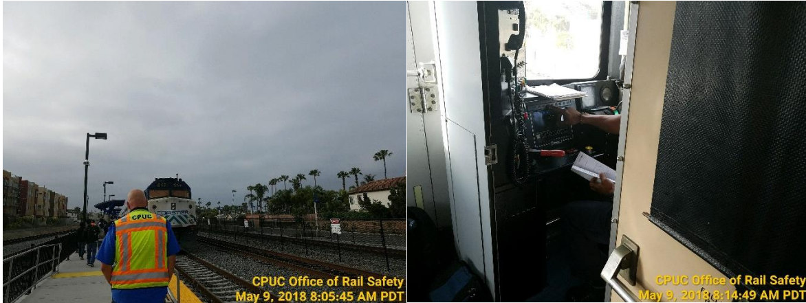
A CPUC inspector is preparing to board a NCTD Coaster passenger train at Oceanside station to observe locomotive engineer operate with PTC. An Engineer is shown initializing the PTC system prior to departure to San Diego Downtown station
