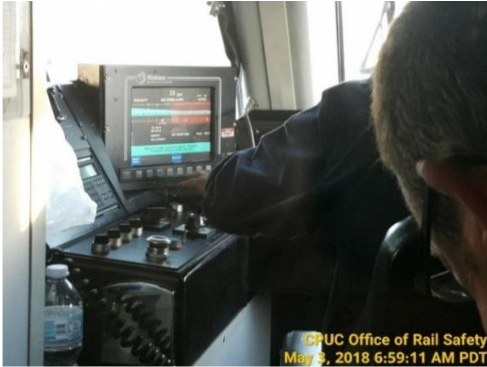
A CPUC inspector observing PTC operations during Metrolink passenger service operations
