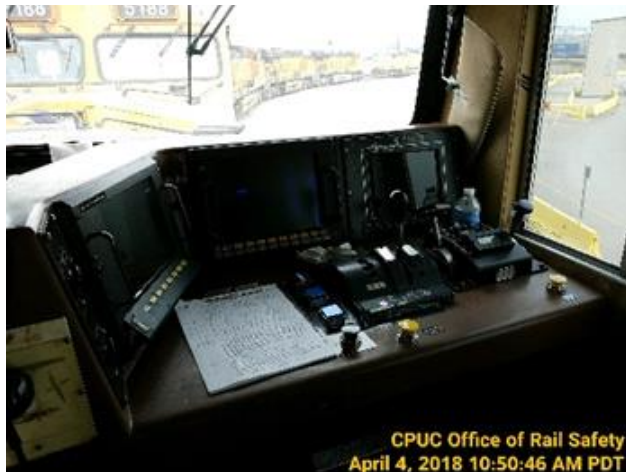
A BNSF Locomotive operating console with PTC screen on the right side
