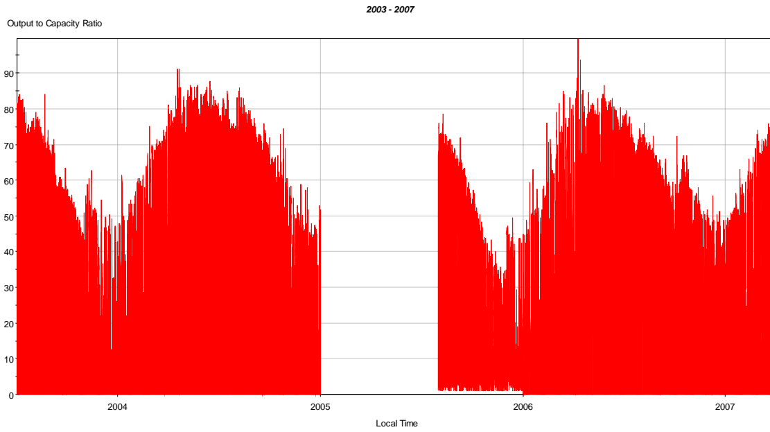
Figure 3-4. Load Profile of a Photovoltaic Cell with Missing Data
