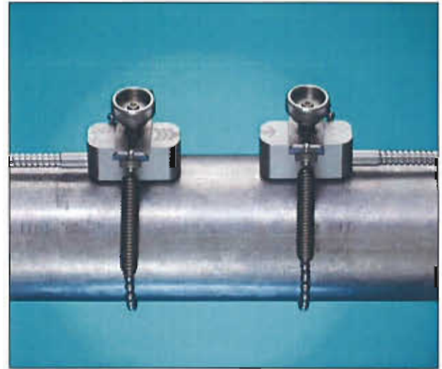
Q3N transducers, mounted with chains
