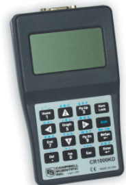
One CR1000KD can be carried from station to station in a CR1000 network.
