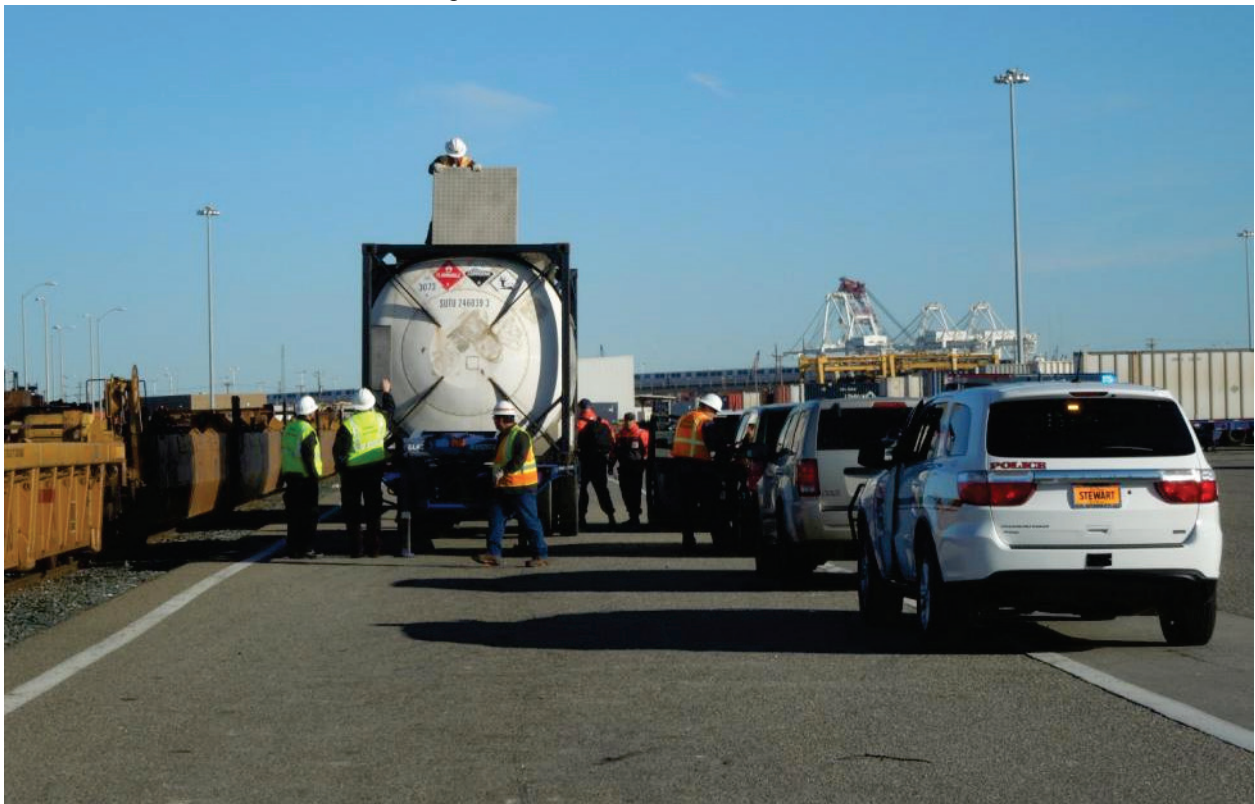
Inspection of an Intermodal Portable Tank Loaded with a Hazardous Material Being Shipped from China to the East Bay area
