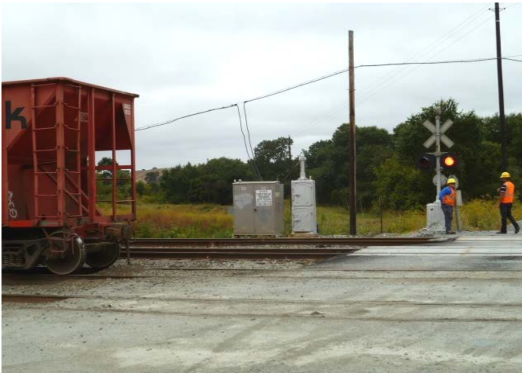
Cars left standing 10 feet from the edge of the roadway at Stonyford private crossing
