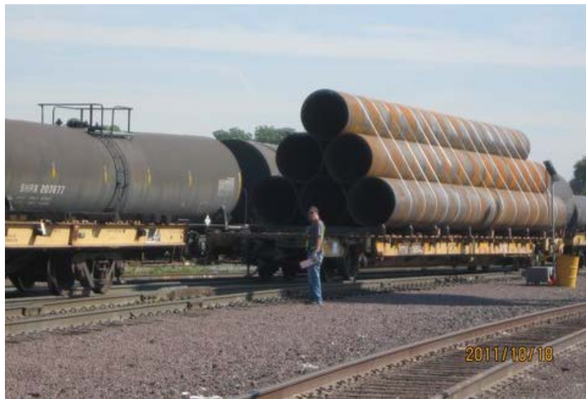
Switchman too close to equipment, and handbrake improperly secured
