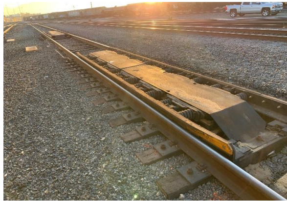
Automatic brake retarder used to stop and hold rail cars at the end of the track.
