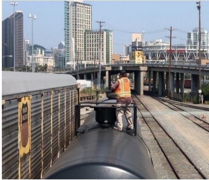
CPUC inspector checking for securement of a tank car containing hazardous material
