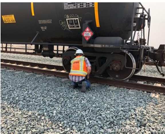
RSD Mechanical inspector checking for proper side bearing clearance underneath the rail car. Improper side bearing clearance may cause the rail car to subsequently derail.
