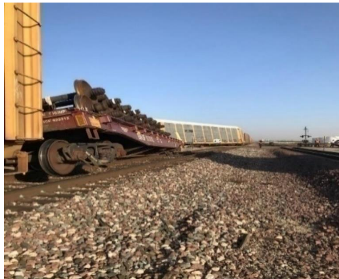
Loaded car placed between two empty cars
