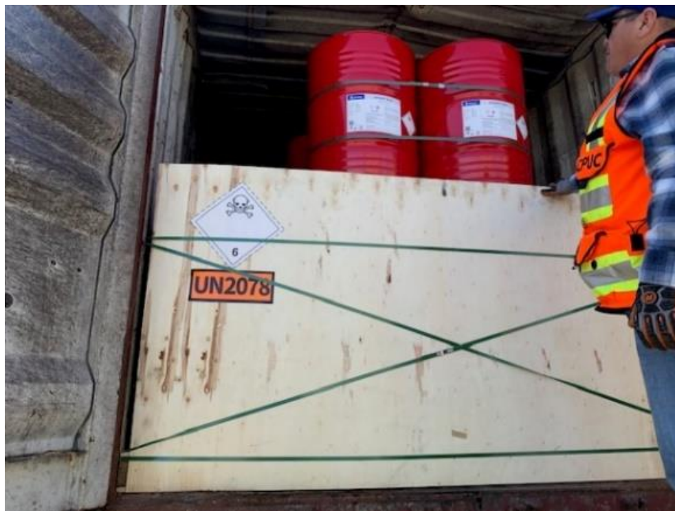
Steel drums loaded on top could potentially fall out when opening the door
