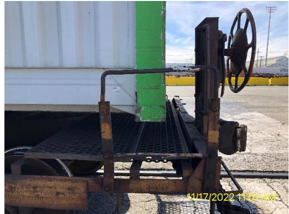
Rail car walkway obstructed by container
