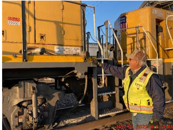
RSD inspector observing a hose laying on a locomotive walkway presenting a tripping hazard
