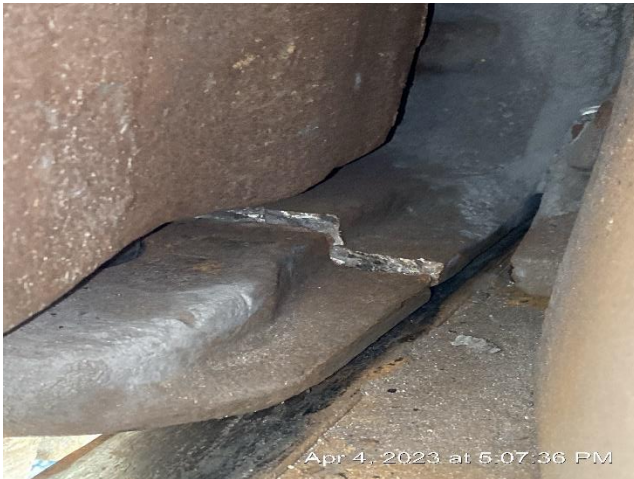
Broken coupler yoke
