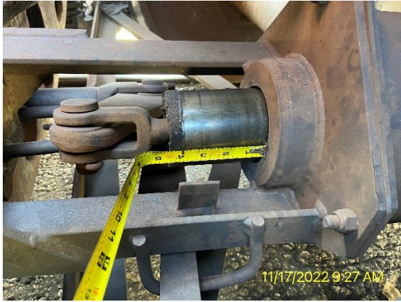
Brake cylinder exceeding required travel limit
