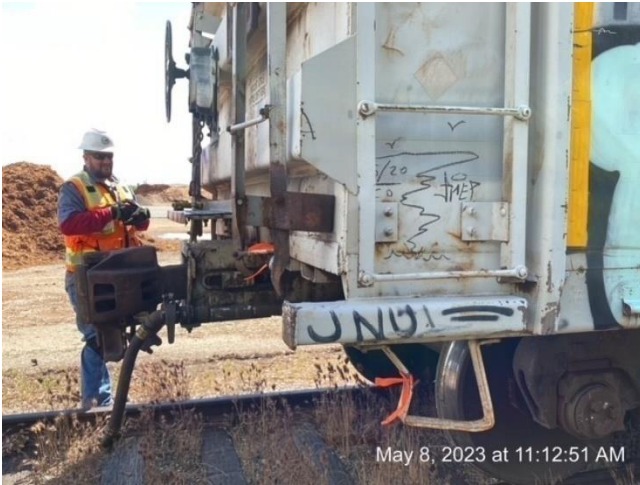
RSD inspector checking coupler
