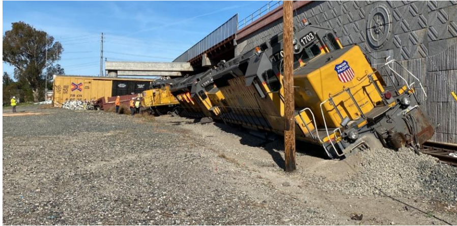
Locomotives and rail cars derailed as result of an uncontrolled movement
