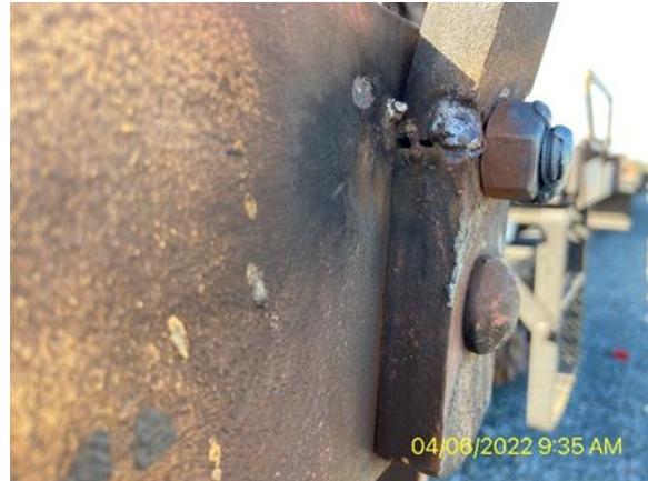
Broken vertical handhold bracket that may further break and cause a railroad employee to fall from the equipment
