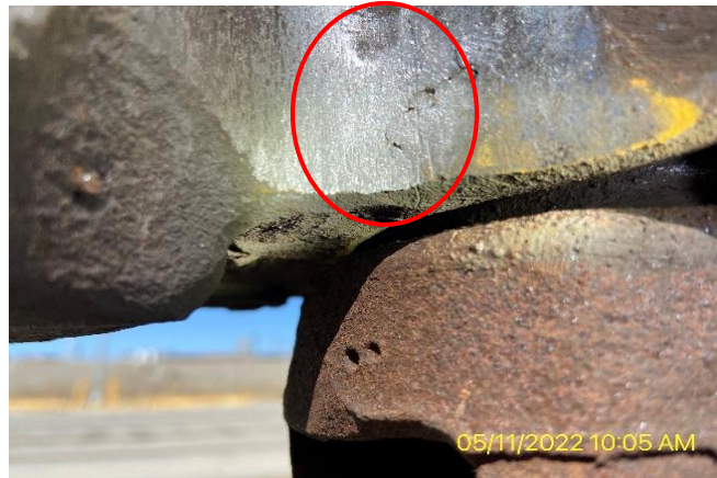
Crack in coupler knuckle
