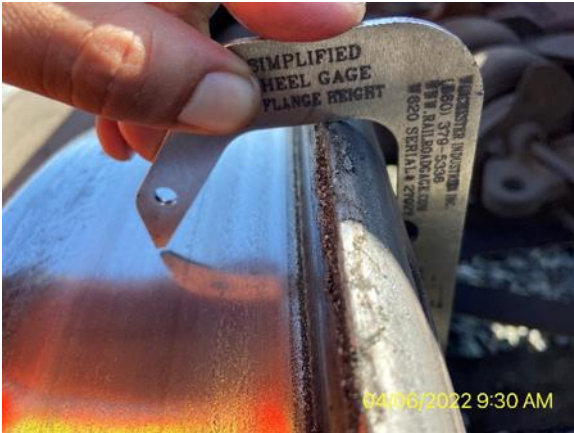
RSD inspector identifying a defective high flange on a rail car wheel, which potentially could cause the rail car to derail
