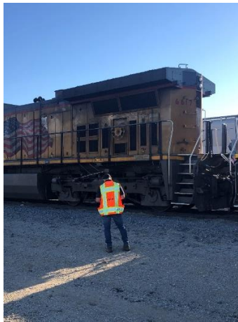
RSD inspector observing UP locomotive to ensure it is secured properly to prevent an uncontrolled movement.
