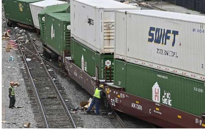
Derailed cars on the crossover switch
