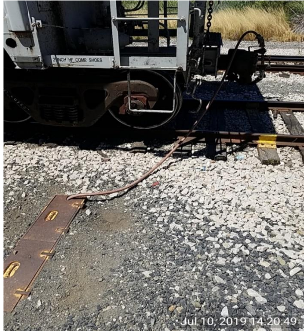
After: Air charging hose position changed to reduce tripping hazard
