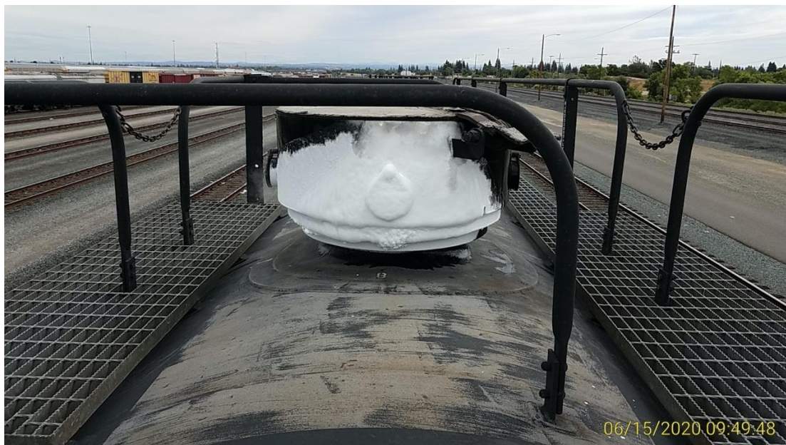
Closeup of ice buildup
