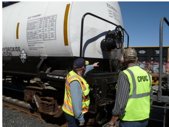
RSD inspectors checking for securement of tank car containing hazardous material
