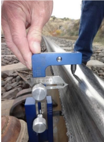
Rail head wear gage used by RSD inspectors
