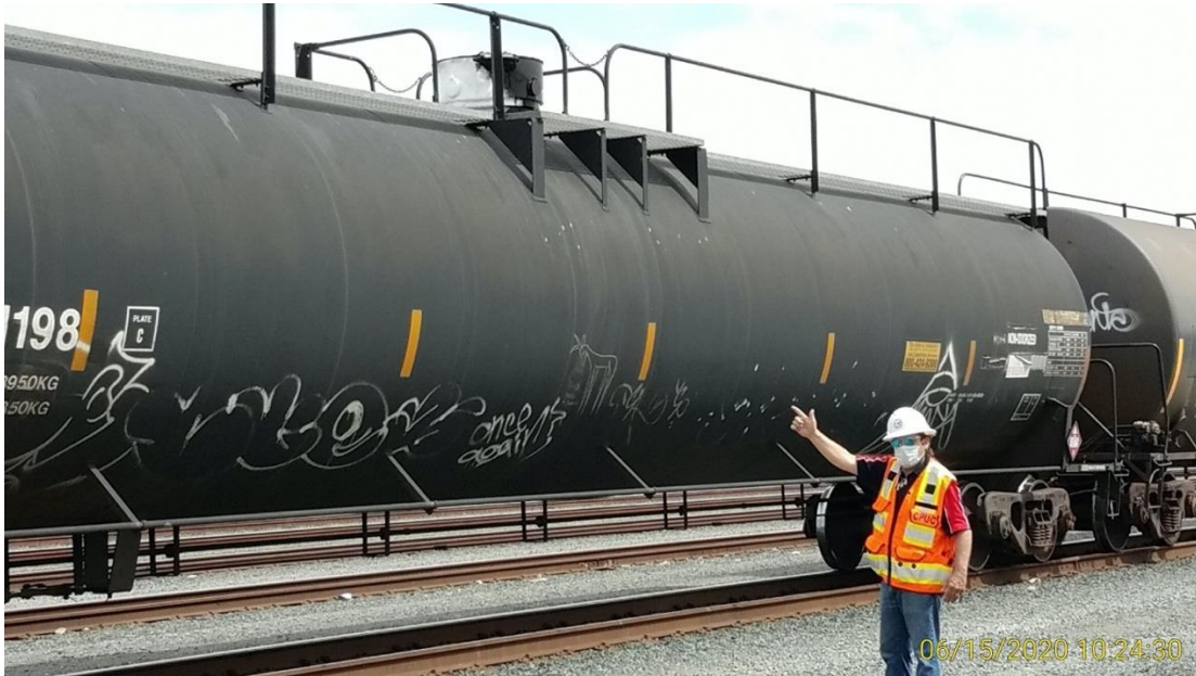
RSD inspector pointing to ice on protective dome of tank car indicating a leak
