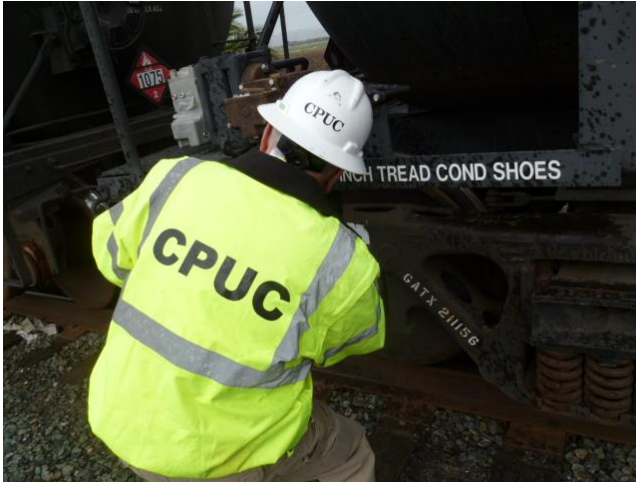
RSD Mechanical inspector checking for the bottom source of a leak in a train's air brake
