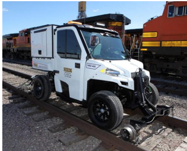
Track testing vehicle equipped with ultrasonic test equipment
